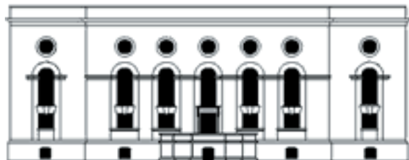
Restored south elevation of the nave with the new steps
